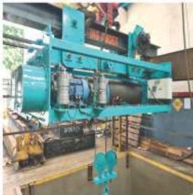
Load Testing upto 50 Ton
